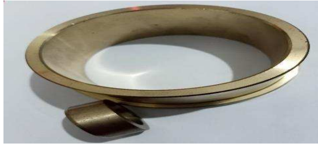
Figure 4 Developed Aluminum bronze bush sleeve
