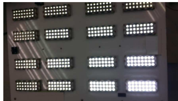
Figure 13. The photograph of the lighting variation of the lower and right sensors
