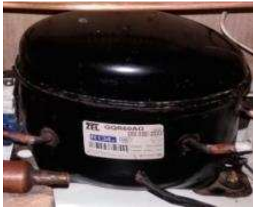
Fig .2The Hermetic type of reciprocating Compressor
