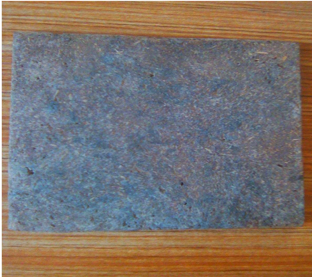
Plate I: Reproduced piliostigma thonningii ceiling board experimental sample
