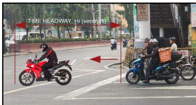
Figure 1.2 Parameters for Time Headway Method (cross-sectional view)
