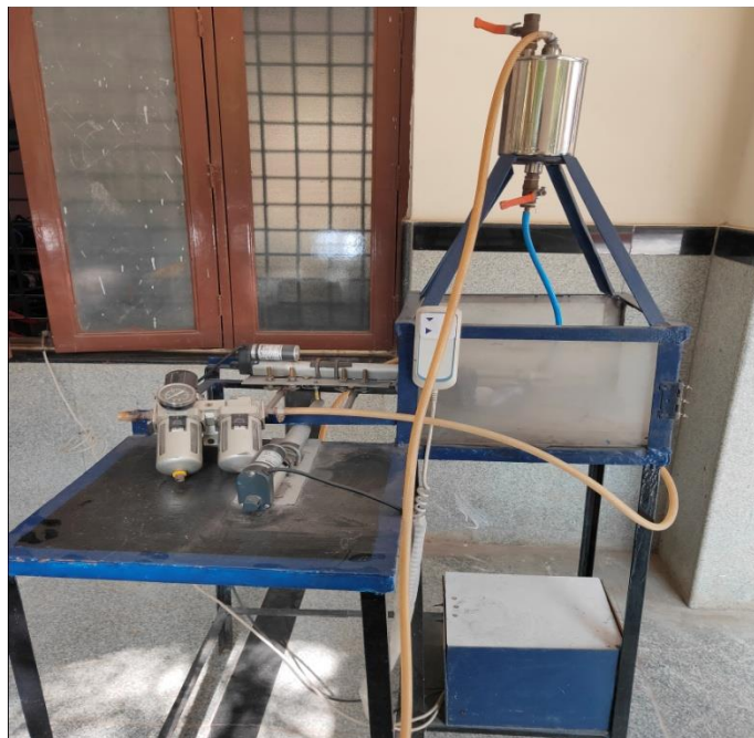
Fig. 2 Abrasive jet machining setup
