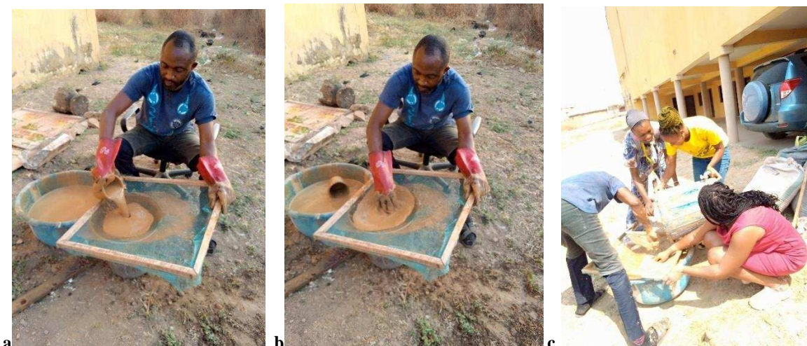
Fig. 3(a); (b) & (c). Process of sieving clay
