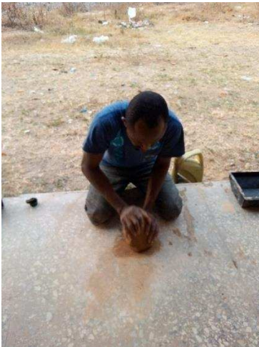
Fig. 4. Kneading of clay
