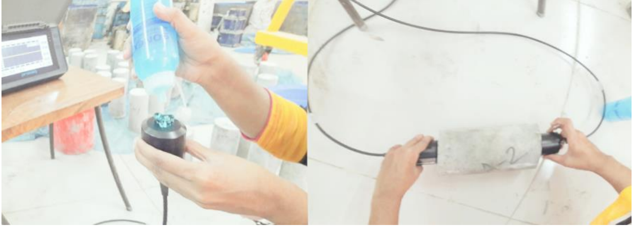
Fig.3: Ultrasonic Pulse Velocity Machine
