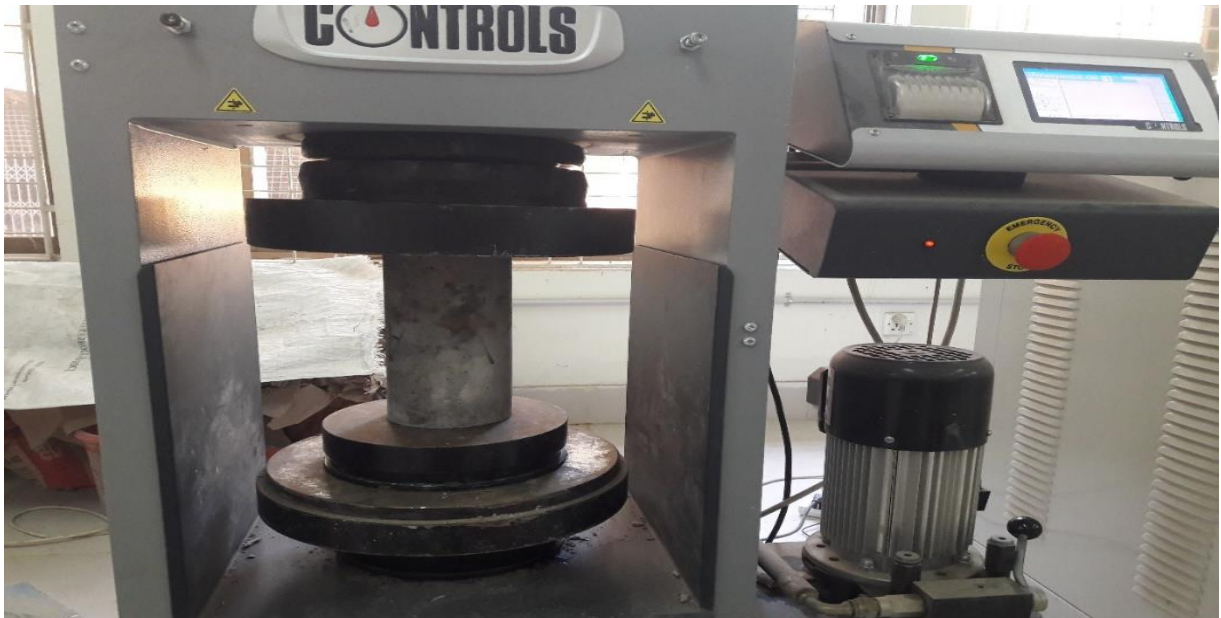
Fig.2. Compression testing machine
