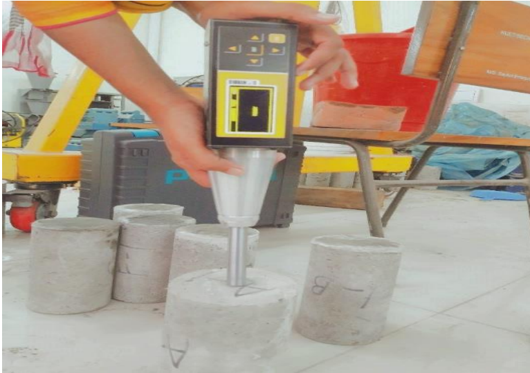
Fig.5: Rebound Hammer Test
