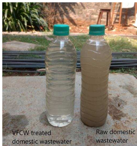
Fig 5. Comparison between VFCW treated and raw domestic wastewater
