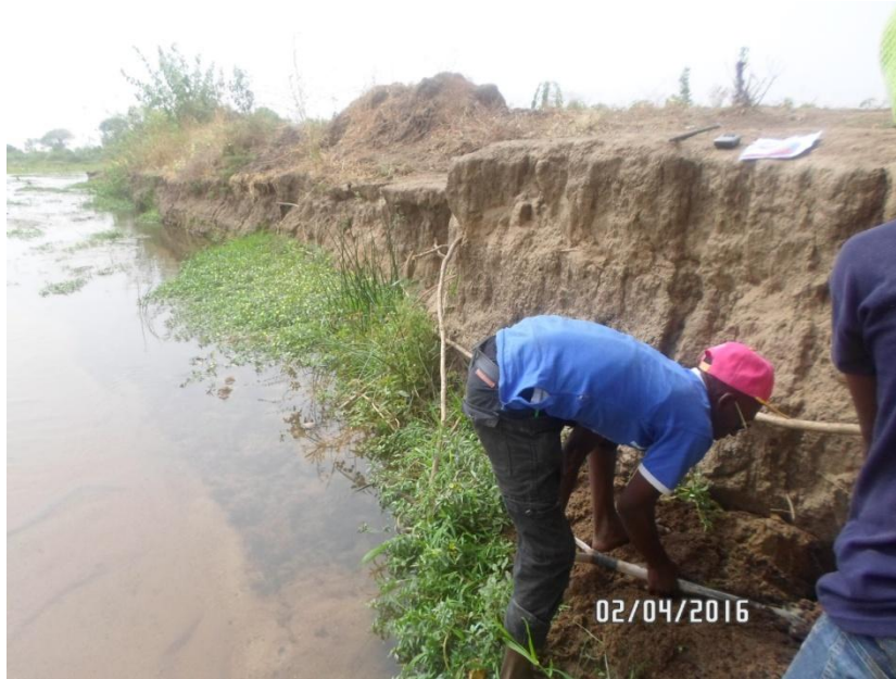
Plate 2: Location 2: Dadinkowa, depth of Gully 4.0m Medium to Coarse Sand
