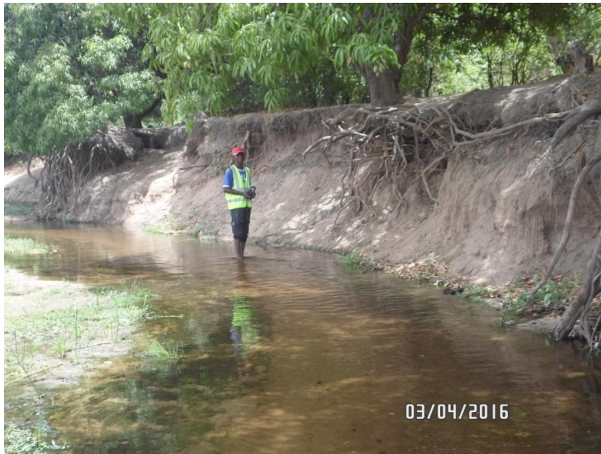
Plate 6: Location 6: Sangereloko depth of gully 2.0m Medium to Coarse sand
