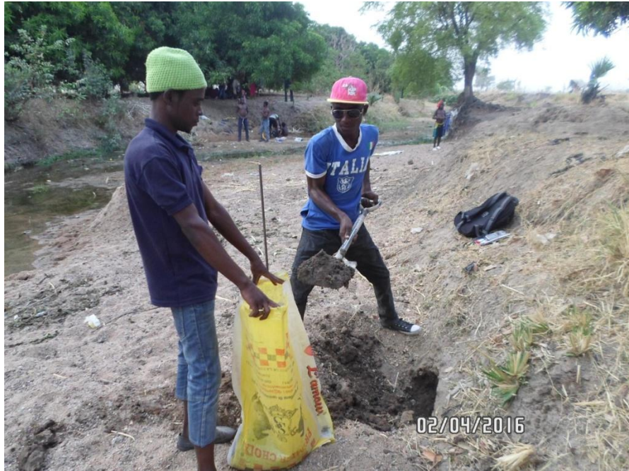
Plate 5: Location 5: Garinlamba depth of gully:1.5m Medium to Coarse sand
