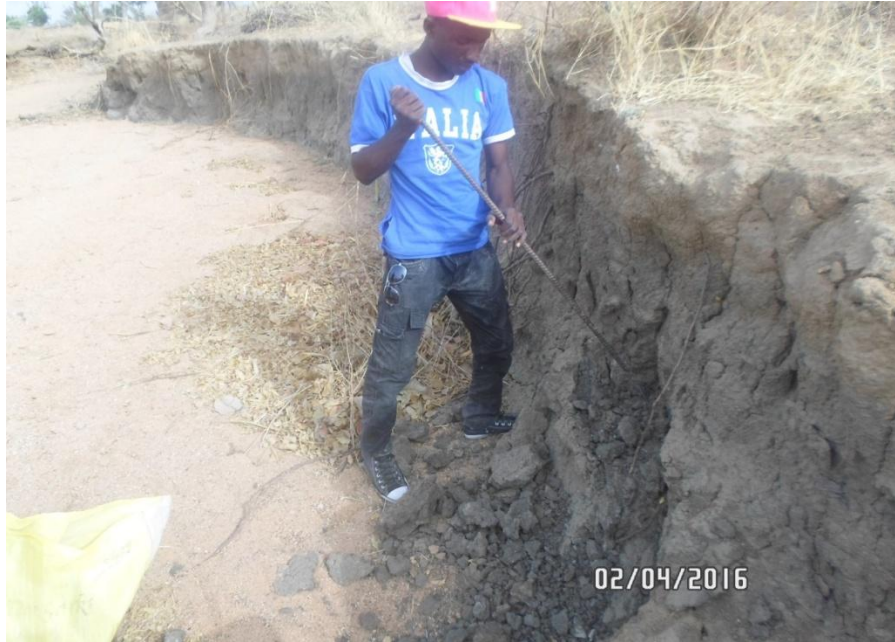
Plate 3: Location 3: Kaulara depth of Gully: 1.3m Medium tp Coarse sand
