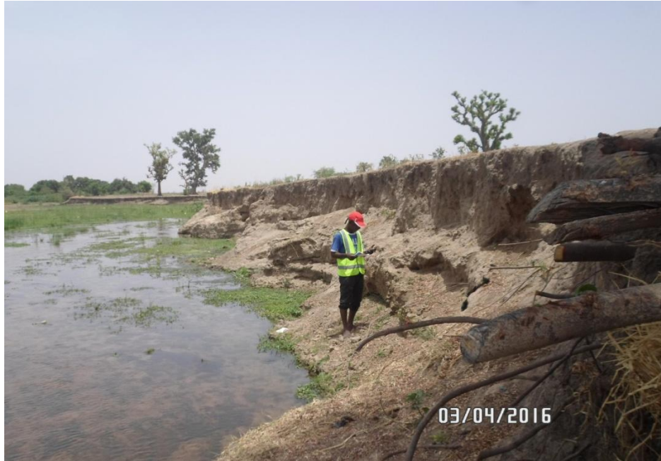
Plate 7: Location 7: Purudomon depth of gully: 6m Medium to Coarse sand
