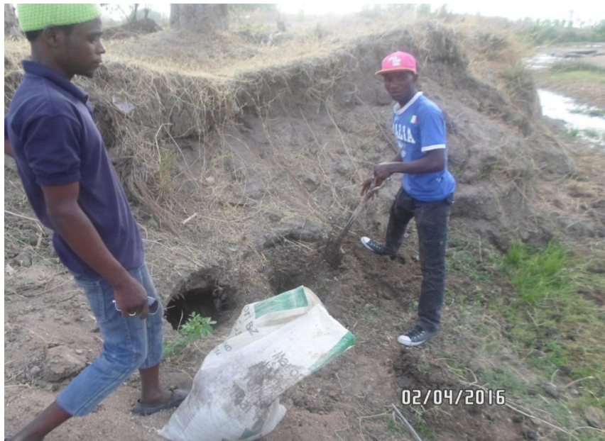
Plate 4: Location 4: Bolki depth of gully: 2.0 m Midium to Coarse sand
